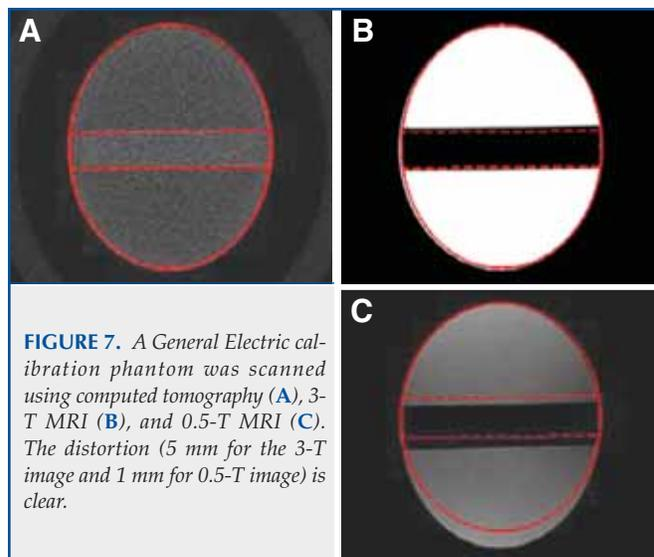
**FIGURE 7.** A General Electric calibration phantom was scanned using computed tomography (**A**), 3-T MRI (**B**), and 0.5-T MRI (**C**). The distortion (5 mm for the 3-T image and 1 mm for 0.5-T image) is clear.
